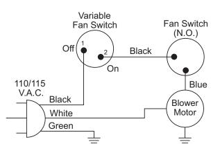
Figure 29 - Blower Wiring Diagram for Thermostat-Controlled Models
